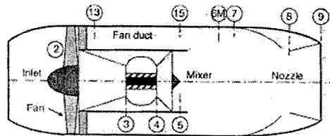
For a mixed exhaust turbofan engine the design parameters are as follows:
