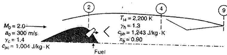
Note that suffix 'c' stands for cold and suffix 'h' stands for hot in the diagram above.  $\pi$  stands for stagnation pressure ratio across an engine component.
