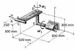
The position of the stylus tip A is controlled by the robot shown. In the position shown the stylus moves at a constant speed u=180 mm/s relative to the solenoid BC. At the same time, arm CD rotates at the constant rate,  $\omega_2=1.6$  rad/s with respect to component DEG. Knowing that the entire robot rotates about the X axis at the constant rate  $\omega_1=1.2 rad/s$ , determine (a) the velocity of A, (b) the acceleration of A.
